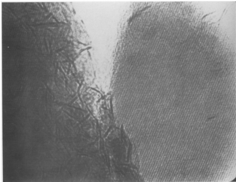
FIG. 3. Transmission electron micrograph of spent Fe-Mo catalyst showing Fe 1-x S and MoS 2 -like phases.
